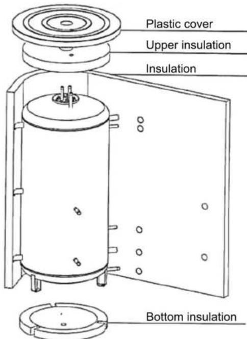
100 mm (1500 l), 120 mm (2000 l) thick insulation NEODUL LB PP. The top cover, covers of flanges and hole caps are integral components. Insulation is supplied in separate packing.
