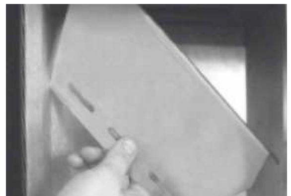
Figure 14. Remove the fire protection plate
