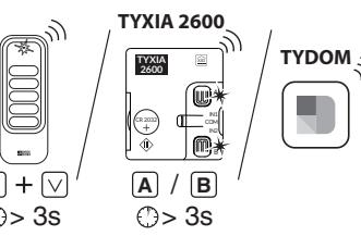
③ When the receiver LED has stopped flashing. The products are now associated.
