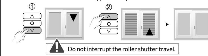
**Note:** The learning for the shutter travel time adjusts itself automatically for each complete cycle from stop to stop.
