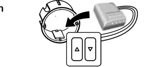
You can install the receiver for roller shutter in a flush-mounted box behind a switch or control push-button or in a sealed box inside the roller shutter, a safe distance from metal parts.
