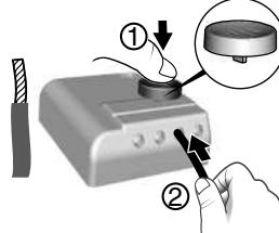
Using the tool supplied or a 2.5 mm screwdriver, press the terminal button then insert the wire.
